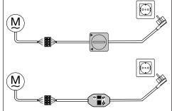
Automatic setting of limit positions is possible, where a stop system is present on both sides, using the rotary switch set (Item no. 4901 001 158 0), a standard rotary switch or the programming unit for drives with electronic limit switching (Item no. 4935 200 011 0). All other functions can only be set via the programming unit.
